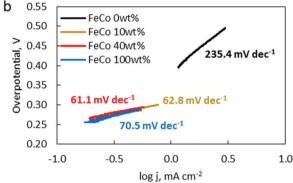
Fig. 9 (a) LSVs of FeCo 0 wt% (black), FeCo 10 wt% (gold) FeCo 40 wt% (red), and FeCo 100 wt% (blue) from 1.0 V to the onset of the OER, in 1.0 M KOH, sat. Ar, at 1600 rpm, at a scan rate of 1 mV  $\rm s^{-1}$ . (b) Tafel slopes derived from polarisation curves in (a). Overpotential is calculated from the thermodynamic potential of the OER (1.23 V vs. SHE).
