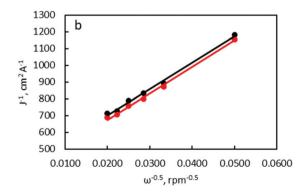
Fig. 11 (a) LSV of FeCo 40 wt% at a RDE rotation speed of 400 rpm (dark red), 900 rpm (red), 1225 rpm (yellow), 1600 rpm (light green), 2025 rpm (green) and 2500 rpm (blue). (b) A K-L plot of polarisation curves from LSV at 0.45 (red) and 0.50 V (black).
