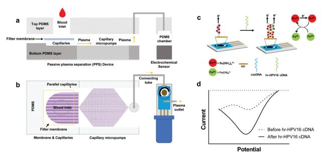
Fig. 1 Overview and working mechanisms of IMEAC. Side view (a) and top view (b) of the IMEAC device that integrates two main modules: PPS for plasma isolation and an electrochemical biosensor. (c) Working principle of the electrochemical sensor for hr-HPV16 cDNA detection. (d) A sample graph extracted from IMEAC showing the presence of hr-HPV cDNA in the extracted plasma sample.
