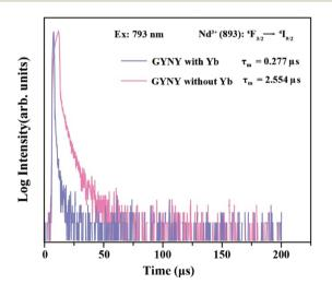
Fig. 4 Luminescence decay curves of  ${\rm Nd}^{3+}$  emissions measured at 893 nm for GYNY with and without  ${\rm Yb}^{3+}$  nanocrystals by pulsed 793 nm excitation.
