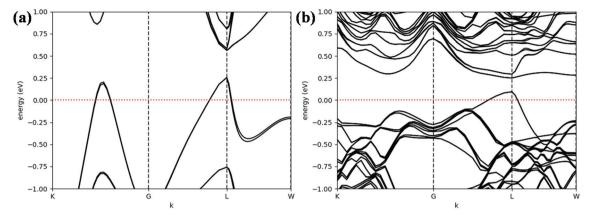
Fig. 5 (a) Electronic band structure of cubic GeTe and (b) cubic Ge<sub>0.9</sub>Sb<sub>0.1</sub>Te.
