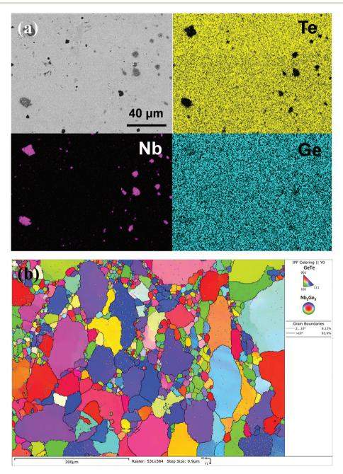
Fig. 2 (a) SEM (scanning electron microscopy) EDS (energy-dispersive X-ray spectroscopy) of the GeTe-Nb₅Ge₃ nanocomposite sample showing Nb-rich regions and Te-poor regions, providing clue of Nb<sub>x</sub>Ge<sub>y</sub> phase in GeTe matrix. (b) EBSD (electron backscatter diffraction) mapping showing large grain sizes, with small Nb<sub>5</sub>Ge<sub>3</sub> precipitates within the grains.
