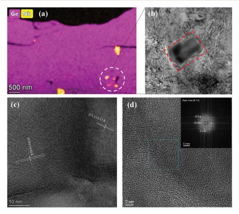
Fig. 3 (a) TEM (transmission electron microscopy) EDS image showing Nb<sub>5</sub>Ge<sub>3</sub>, phase embed in GeTe matrix. (b) Zoom in image showing Nb<sub>5</sub>Ge<sub>3</sub>. (c) HRTEM image showing (100) and (211) lattice spacing of Nb<sub>5</sub>Ge<sub>3</sub>. (d) HRTEM with SAED (selected area electron diffraction) in inset.
