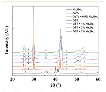
Fig. 1 XRD patterns of pristine GeTe, Nb<sub>5</sub>Ge<sub>3</sub>, Ge<sub>0.9</sub>Sb<sub>0.1</sub>Te (GST), and GST-Nb<sub>5</sub>Ge<sub>3</sub> nanocomposites with different wt%. \* denotes Ge precipitates peaks, # denotes Nb<sub>5</sub>Ge<sub>3</sub> peaks.
