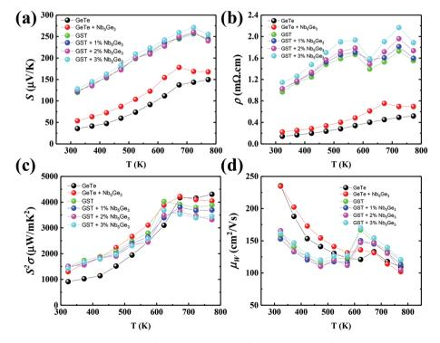
Temperature dependent (a) Seebeck coefficient (b) electrical resistivity (c) power factor, and (d) weighted-mobility of all samples.
