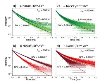
Fig. 7 UC luminescence decay curves for (a), (c)  $\beta$ - and (b), (d)  $\alpha$ -NaGdF $_4$  UCNPs of two different sizes (S/V as labeled in the figure) dispersed in toluene monitoring either the UCNPs' green ( $\lambda_{em}$  = 550 nm) or red ( $\lambda_{em}$  = 650 nm) emission following 980 nm excitation. From these decay curves, respective excited state lifetimes have been determined using a Kohlrausch fitting function (solid lines).
