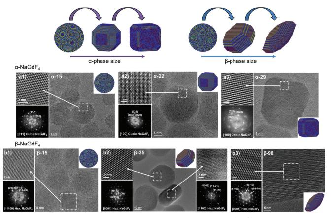
Fig. 2 HRTEM images, SAED patterns and morphological models of selected (a)  $\alpha$ - and (b)  $\beta$ -NaGdF<sub>4</sub>:Er<sup>3+</sup>/Yb<sup>3+</sup> UCNPs (additional data available in Fig. S2†).
