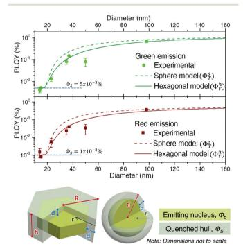
Fig. 5 β-NaGdF<sub>4</sub> experimental PLQY data (green emission on top, red emission below) fitted to a simple nucleus/hull volumetric model assuming spherical (dashed lines) and hexagonal particles (full line). A scheme of the two shapes indicating the different parameters used for their definition is given below the graphs.
