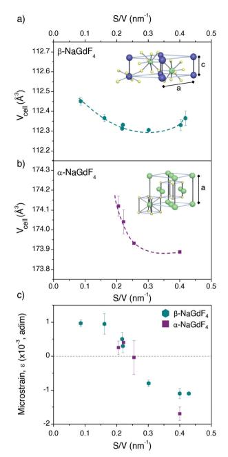
Fig. 6 Unit cell volume calculated from the lattice parameters given in Table 2 and plotted *versus* the S/V ratio for (a)  $\beta$ - and (b)  $\alpha$ -NaGdF<sub>4</sub> UCNPs. Schemes depicting the ion positions within each unit cell are given as insets. (c) Microstrain parameters obtained for each sample as a function of S/V.
