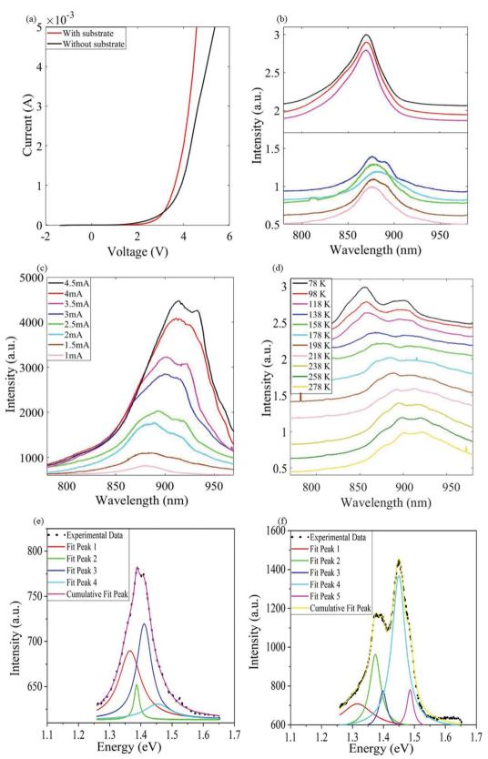
Fig. 4 (a) I-V characteristics of the on-substrate and flexible devices. (b) Room temperature PL spectrum at different positions on the array for onsubstrate (top) and flexible devices (bottom). (c) EL spectrum of the flexible device at room temperature at different current injection levels. (d) Temperature dependent EL spectrum at a 1 mA current from the flexible LED. Lorentz curve fitting of the EL spectrum measured at 1 mA at (e) room temperature and (f) 78 K.
