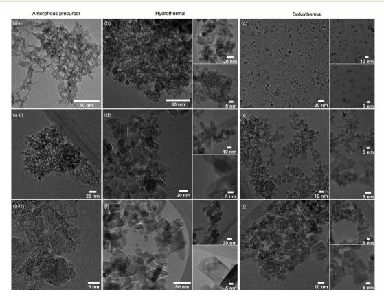
Fig. 2 TEM images of undoped amorphous titania precursor (a(i-iii)), and undoped titania treated for 24 hours hydrothermally and solvothermally, respectively, at  $100 \,^{\circ}\text{C}$  (b and c),  $150 \,^{\circ}\text{C}$  (d and e), and  $200 \,^{\circ}\text{C}$  (f and g). Insets show the corresponding higher magnification images and HRTEM where possible.
