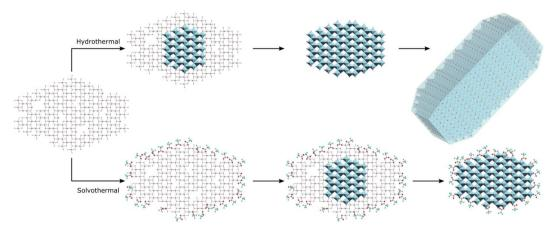
Scheme 1 Hydrothermal treatment of amorphous titania leads to intraparticle crystallisation of the anatase phase and subsequent growth by interparticle fusion, while solvothermal treatment in trifluoroacetic acid initially leads to complete surface modification with intraparticle crystallisation yielding surface capped anatase phase hybrid nanocrystals.
