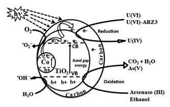
Fig. 11 Photocatalytic reduction of the  $U(v_i)$ -ARZ3 mechanism using C@TiO<sub>2</sub>-C under UV light.
