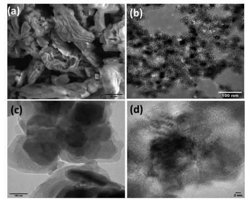
Fig. 2 SEM (a) image and TEM image (b-d) of the synthesized Co@TiO<sub>2</sub>-C photocatalyst.
