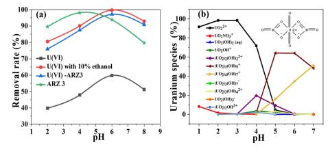
Fig. 5 (a) The effect of pH on the degradation/reduction of 50 mg  $L^{-1}$  U(vi)-ARZ3, free ARZ3 dye, and free U(vi) ions using the Co@TiO2-C photocatalyst for 60 min (solution volume; 10 mL, catalyst weight; 10 mg) and (b) speciation of uranium in aqueous solution at different pH values.
