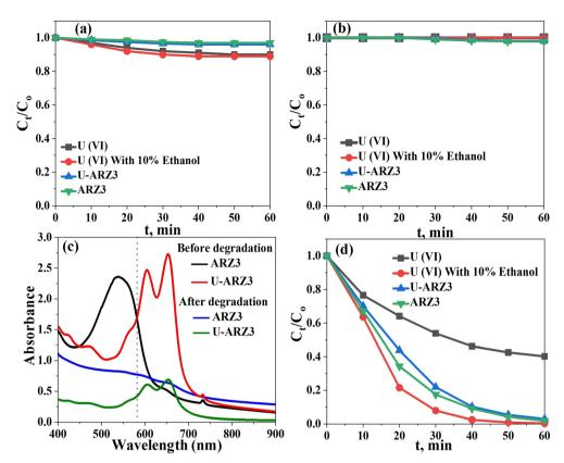
Fig. 4 (a) Effect of UV light on U(vı) and ARZ3 solutions without Co@TiO $_2$ -C catalyst. (b) Effect of Co@TiO $_2$ -C in the dark. (c) Effect of Co@TiO $_2$ -C in UV light. (d) Absorbance spectra of ARZ3 and the U(vı)-ARZ3 complex.
