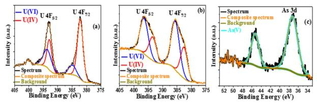
Fig. 9 (a) U 4f XPS spectra in 10% ethanol and (b and c) U 4f and As 3d XPS spectra of the U(v)-AZR3 complex.
