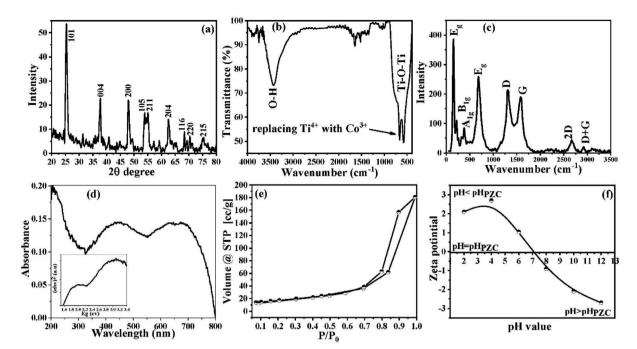
Fig. 1 (a) XRD patterns, (b) FTIR spectrum, (c) Raman spectrum, (d) UV-vis spectroscopy, (d inset) the energy bandgap, (e)  $N_2$  adsorption/desorption isotherm, and (f) zeta potential in 0.01 M KCl as a function of pH of the synthesized Co@TiO<sub>2</sub>-C photocatalyst.
