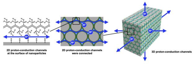
Scheme 1 Schematic model of proton-conductive core-shell type nanoparticle-filled PEM.
