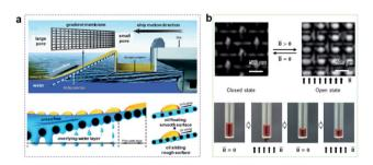
Fig. 5 (a) Inspired by fish gills, a hydrophilic gradient membrane can be used for oil-water separation. 105 Adapted with permission from ref. 105. Copyright 2017, American Chemical Society. (b) Controllable penetration of liquid by a magnetically responsive micro/nano porous composite membrane. 118 Adapted with permission from ref. 118. Copyright 2022, Royal Society of Chemistry.
