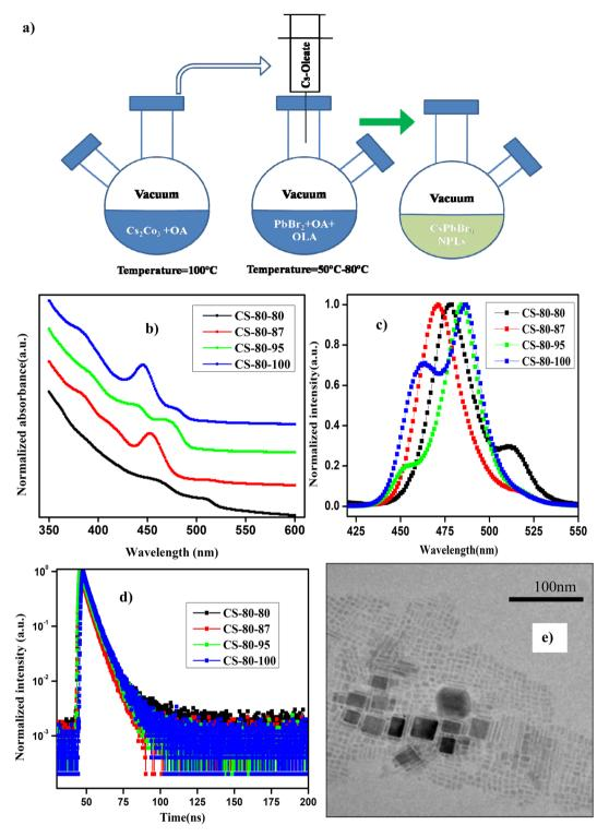
Fig. 1 (a) Schematic diagram of the synthesis process of perovskite nanoplatelets using the vacuum-assisted low-temperature (VALT) method. (b) UV-visible absorption and (c) normalized PL spectra of the NPLs that were synthesized at 80 °C. (d) TRPL decay curves of the NPLs synthesized at 80 °C with different preheating temperatures for the PbBr<sub>2</sub> precursor. (e) TEM image of the sample CS-80-95.
