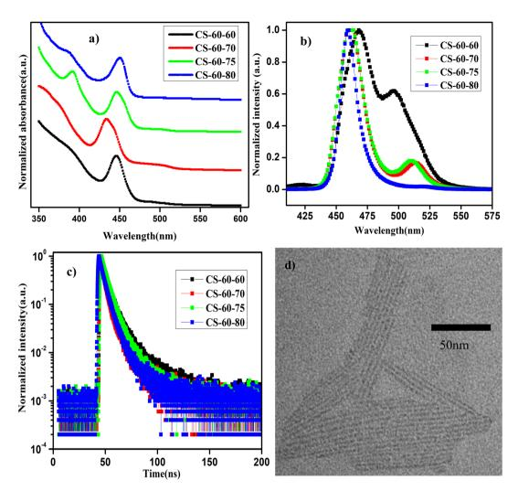
Fig. 3 (a) UV-visible absorption and (b) normalized PL emission spectra of the NPLs synthesized at 60 °C with different PbBr<sub>2</sub> precursor temperatures. (c) TRPL decay curves for the NPLs synthesized at 60 °C under different conditions. (d) TEM image of the sample CS-60-80.
