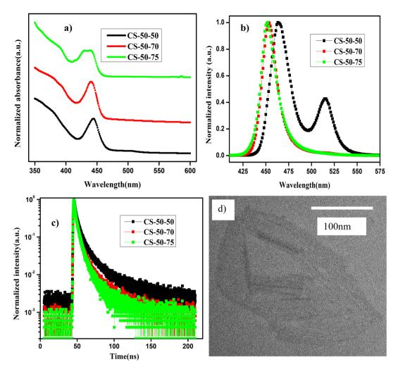
Fig. 4 (a) UV-visible absorption and (b) normalized PL emission spectra of NPLs that are synthesized with different preheating temperatures for the PbBr<sub>2</sub> precursor. (c) TRPL decay curves for the NPLs synthesized at 50 °C under different conditions. (d) TEM image of the sample CS-50-70.
