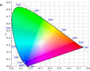
Fig. 5 Comparison of the EL spectra of the thin-film and the PL spectra of the NPL dispersion in hexane (top). Inset shows a photographic image of the fabricated LED. (b) CIE coordinates for the EL spectrum.
