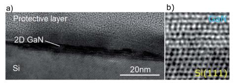
Fig. 4 (a) STEM image of the cross-sectional lamella of an amorphous gallium droplet and crystalline GaN on the Si(111)  $7 \times 7$  substrate. (b) Zoomed-in STEM image of the 2D GaN-Si(111)  $7 \times 7$  interface.
