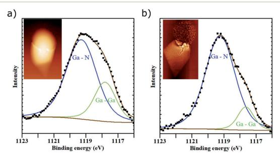
Fig. 2 Fitted XPS Ga  $2p_{3/2}$  peak obtained during the post-nitridation after (a) 60 min and (b) 120 min. The Ga-Ga component is at 1117.8 eV (green curve) and the Ga-N component at 1119.3 eV (blue curve).
