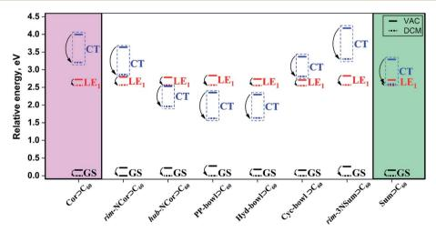
Relative energies (in eV) of GS,  $LE_1$ , and CT states for the complexes of interest computed in a vacuum (VAC) and dichloromethane (DCM).
