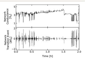
**Fig. 3** Top: Measured conductance of a percolating NP network without matrix upon constant voltage application of 5 V. (2 h extract from the overall measurement). The representation is given in conductance units of  $G_0$  for convenience ( $G_0 = 2e^2/h = 7.748 \times 10^{-5}$  S). The dynamics corresponds to transitions between different metastable states in the network. Bottom: Temporal sequence of network transition events extracted from the upper panel.
