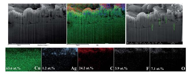
FIB-SEM images and elemental mapping of Aq-electrocatalyst after CO<sub>2</sub>RR at -1.6 V vs. Aq/Aq<sup>+</sup> for 70 min.
