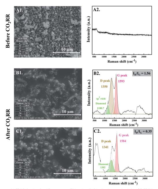
Fig. 1 SEM images with EDX (Left column) and Raman spectra (Right column) of the Ag-electrocatalyst before  $CO_2RR$  (A1 and A2) and after  $CO_2RR$  at ambient conditions for 10 min (B1 and B2) and 20 min (C1 and C2).
