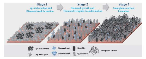
Scheme 1 Evolution of nanostructured Ag-carbon films under room temperature CO<sub>2</sub>RR system.
