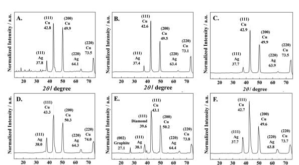
GI-XRD results of (A) Ag-electrocatalyst before CO<sub>2</sub>RR and Ag-electrocatalyst after CO<sub>2</sub>RR for (B) 10, (C) 20, (D) 30, (E) 70, and (F) 140 min.
