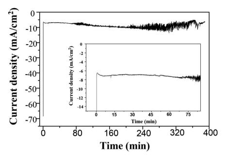
Fig. 10 Total current densities of the Ag-electrocatalyst after CO<sub>2</sub>RR for 390 min.
