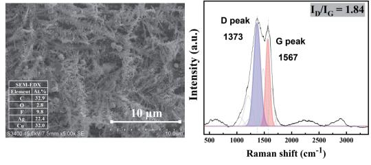
Fig. 11 SEM images (Left column), and Raman results (Right column) of Ag-electrocatalyst after CO<sub>2</sub>RR at ambient conditions for 390 min.
