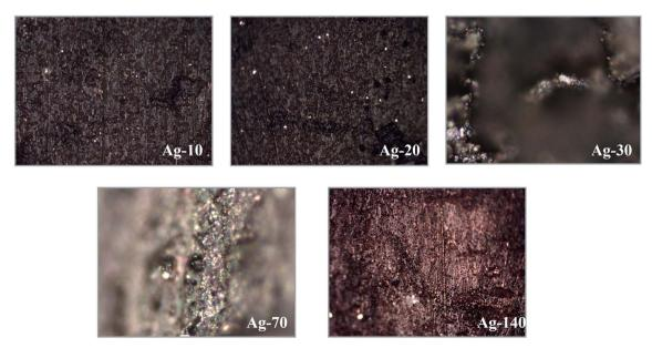
Fig. 9 The optical microscopy images (10×) of Aq-electrocatalyst after CO<sub>2</sub>RR for 10, 20, 30, 70, and 140 min.
