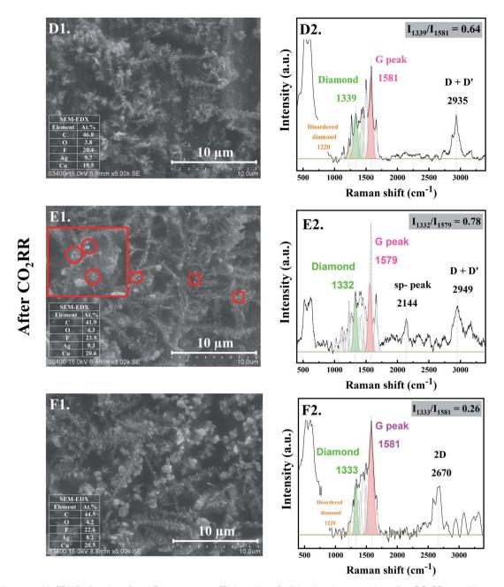
Fig. 2 SEM images with EDX (Left column) and Raman spectra (Right column) of the Ag-electrocatalyst after  $CO_2RR$  at ambient conditions for 30 min (D1 and D2), 70 min (E1 and E2), and 140 min (F1 and F2).
