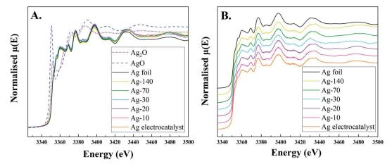
Fig. 7 Normalized XANES spectra at Aq L<sub>3</sub>-edge of Aq-electrocatalyst before and after CO<sub>2</sub>RR for 10, 20, 30, 70, and 140, Aq foil, AqO, and Aq<sub>2</sub>O.
