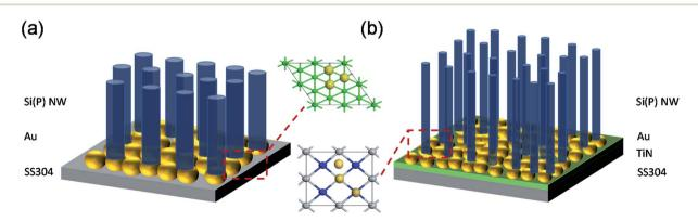
Scheme 1 Schematic representation of Si(P) NWs grown on 3 nm-thick Au/SS304 disks (a) and 3 nm-thick Au/50 nm-thick TiN/SS304 disks (b).
