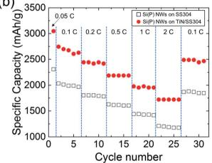
Fig. 5 Specific gravimetric capacities of Si(P) NWs grown on SS304 (black, square, empty) and on TiN/SS304 (red, circle, solid) over cycling at 800 mA  $\rm g^{-1}$  (0.2C for Si) (a) and at different charging rates (b).
