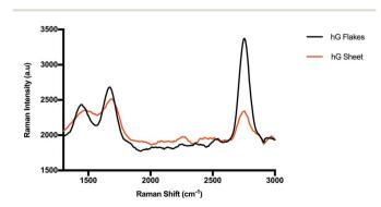
Fig. 7 Raman spectra of hG flakes and an hG sheet.
