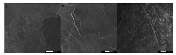
Fig. 3 SEM micrographs of etched AgNP-decorated graphene after (a and b) sonication for 6 h, and (c) mechanical agitation for a week.
