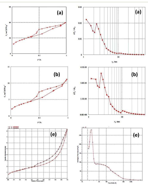
Fig. 4  $N_2$  adsorption—desorption isotherms of PMAMOSa,b,e (1) obtained using the PMDADA precursor I prepared in THF (a) or DMF solvent (b) with the simultaneous addition of precursor I and TEOS to the mixture of HCl and Pluronic P123. CTAB was dissolved in ammonia solution and used as the template (e).
