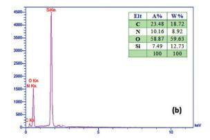
EDX spectra of the obtained PMAMOS using precursor I prepared in THF (a) and DMF solvents (b).
