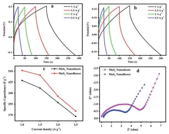
Fig. 7 GCD curve of the (a)  $MoS_2$  nanosheets, (b)  $MoS_2$  nanoflower. (c)  $MoS_2$  nanosheets and  $MoS_2$  nanoflower current density *versus*  $C_{sp}$ , and (d) Nyquist plot of the  $MoS_2$  nanosheets and  $MoS_2$  nanosheets and  $MoS_2$  nanosheets.
