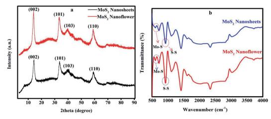
Fig. 1 (a) XRD pattern of the MoS<sub>2</sub> nanosheets and MoS<sub>2</sub> nanoflower. (b) FT-IR spectra of the MoS<sub>2</sub> nanosheets and MoS<sub>2</sub> nanoflower.
