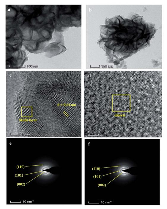
Fig. 3 HR-TEM images of the (a) MoS<sub>2</sub> nanosheets, (b) MoS<sub>2</sub> nanoflower, and (c and d) HR-TEM high resolutions images, (e and f) SAED pattern of MoS<sub>2</sub> nanosheets and MoS<sub>2</sub> nanoflower.
