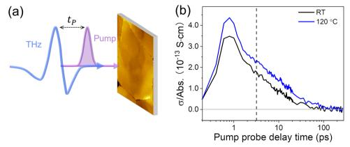
Fig. 4 (a) Schematic of optical-pump THz-probe spectroscopic studies on the perovskite sample supported by SiO2; (b) comparison of photoconductivity  $\sigma$  normalized to the absorbed photon density ( $N_{abs}$ ) for RT and 120 °C deposited (TEA)<sub>2</sub>SnI<sub>4</sub> perovskite films.
