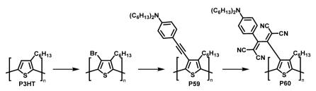
Fig. 25 Post-polymerisation functionalisation of P3HT: halogenation followed by Stille coupling for the synthesis of P59 and subsequent reaction with TCNE giving P60.114
