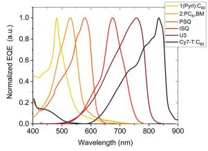
Fig. 5 Normalized EQE of OPDs based on narrow-photo-absorbing materials as a function of wavelength.  $1(Pyrl):C_{60}^{177}$  and  $Cy7-T:C_{60}^{22}$  are PHJs. 2:PC<sub>61</sub>BM<sup>21</sup> is a BHJ blend. PSQ<sup>19</sup> and ISQ<sup>20</sup> are single-component photo-absorbing materials with D-A-D chemical structure and U3 is also single component device.23
