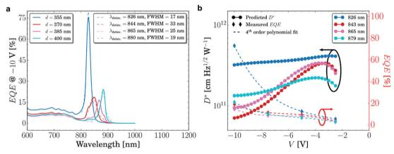
Fig. 13 (a) Amplified EQE of narrowband CT-PM-OPD at four resonance wavelengths at -10 V. (b) EQE and  $D^*$  of the same devices shown in (a) at various voltages.<sup>201</sup> Licensed under CC BY 4.0.
