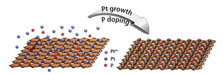
Fig. 1 Fabrication process of phosphorus-modified Pt@Cu (Pt/P@Cu).
