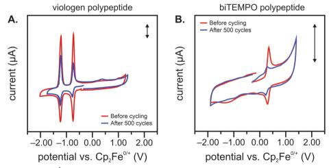
Fig. 5 Cyclic voltammetry at 100 mV s $^{-1}$  of the (A) viologen polypeptide anolyte and (B) biTEMPO polypeptide catholyte before and after cycling of the polypeptide redox flow cell (arrows denote 10  $\mu$ A). Glassy carbon was used as the working electrode, platinum wire as the counter electrode, un-fritted freshly anodized Ag/AgCl wire as the reference electrode, and ferrocene was used as internal reference. The supporting electrolyte was 0.5 M TEATFSI in ACN.
