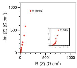
**Fig. 3** Nyquist plot of the EIS data before galvanostatic cycling for the redox flow cell with a BiTEMPO polypeptide catholyte and viologen polypeptide anolyte. EIS was conducted with circulating electrolytes at open circuit potential with an amplitude of 10 mV in a frequency range of 200 kHz to 0.4 Hz (5 steps per decade).
