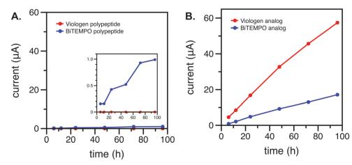
Fig. 2 Crossover study of (A) viologen and biTEMPO polypeptides and (B) their small-molecule analogs using an FAPQ 375 PP membrane. The currents were taken as the averages of absolute values of the CV anodic and cathodic peak currents over time for the blank electrolyte side of the H-cell.
