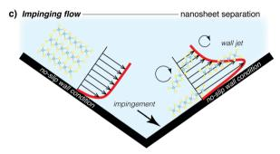
Fig. 12 Microfluidisation of nanosheets from layered materials. The synthesis mechanisms depend on the hydrodynamic regime and chamber configuration. Production of nanosheets can be achieved through (a) laminar or viscous shear exfoliation, (b) turbulent shear exfoliation and/ or (c) localised flow impingement.
