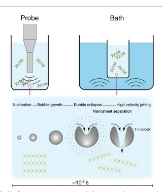
Fig. 11 Sonication-based synthesis typically involves either probe or bath techniques. Exfoliation of layered materials into nanosheets is achieved through the rapid growth and collapse of cavitation bubbles in the liquid dispersion.
