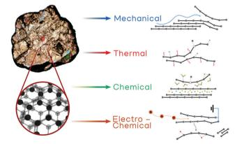
Fig. 9 Schematic representation of the different exfoliation techniques discussed in this review: liquid-phase "mechanical", thermal, chemical and electro-chemical exfoliation
