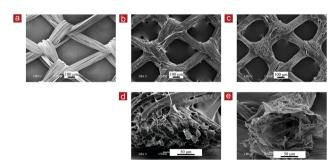
Fig. 3 SEM images of the top surface view (a-c) and the cross-sectional view (60° view) (d and e) of the PLGA mesh (a), collagen-coated PLGA mesh (b and d) and collagen mesh-L (c and e).
