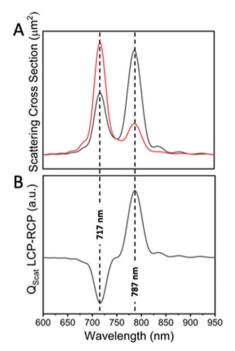
Fig. 2 Circular dichroism spectra of dimer-1 emerging from the difference between the scattering of LCP (black) and RCP (red) light (A) giving rise to a bisignate form of the spectrum (B).
