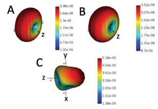
**Fig. 4** Calculated far-field profiles of the gold nanorod dimer-1. (A) Dimer excited by LCP light at the anti-bonding wavelength of 709 nm, and at the bonding wavelength of 774 nm (B). (C) Off-resonance excitation at 650 nm of the gold nanorod dimer.
