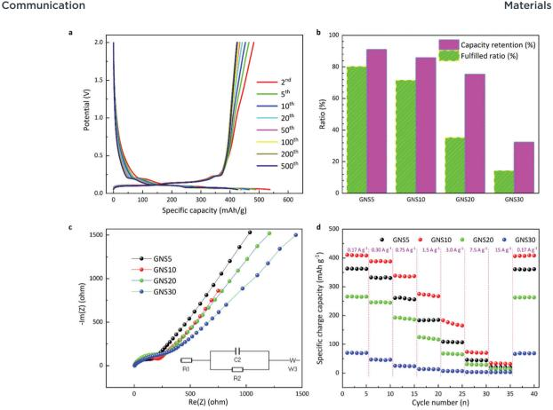
Fig. 4 (a) Discharge and charge patterns of GNS10 (0.17 A  $g^{-1}$  within [0.05, 2] V), (b) capacity retention and fulfilled ratio of the cycling performance, (c) the galvano electrochemical impedance spectra of GNS5, GNS10, GNS20, and GNS30 from  $10^6$  to 0.01 Hz at AC = 0.1 mA with the inset equivalent circuit, and (d) rate capability of GNS5, GNS10, GNS20, and GNS30 at various current densities.
