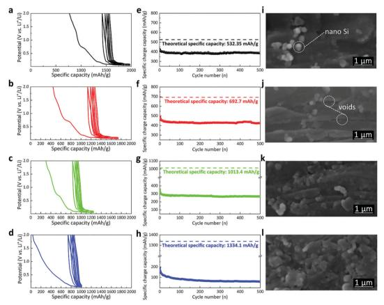
Fig. 3 First five discharge/charge curves (cyclic type) at 0.17 A  $g^{-1}$  (a–d), specific charge capacity with calculated theoretical limits (e–h), and cross-sectional SEM images (i–l) of GNS5 (a, e and i), GNS10 (b, f and j), GNS20 (c, g and k) and GNS30 (d, h and l).
