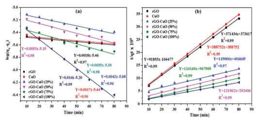
Fig. 12 (a and b) Pseudo first and second-order kinetics plots for EBT on rGO, CuO and CuO/rGO nanocomposites
