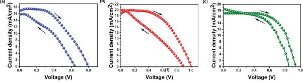
Fig. 5 /-V characteristics of the as-prepared (a) PSC-HTM-free, (b) PSC-spiro and (c) PSC-CuSCN
