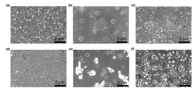
Fig. 3 FESEM morphological images of (a and d) PSC-HTM-free, (b and e) PSC-spiro and (c and f) PSC-CuSCN, under as-prepared (a-c) and aged (d-f) conditions, respectively.
