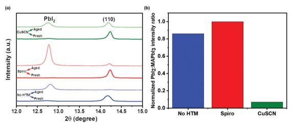
Fig. 4 (a) XRD pattern highlighting the Pbl<sub>2</sub> and (110) peak of MAPbl<sub>3</sub> fresh and aged PSC-HTM-free, PSC-spiro and PSC-CuSCN devices. (b) Normalized Pbl<sub>2</sub>:MAPbl<sub>3</sub> peak intensity ratios of the aged devicess.
