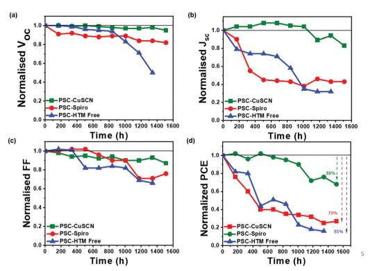
Fig. 6 Normalized (a)  $V_{oc}$ , (b)  $J_{sc}$ , (c) FF and (d) PCE of the PSC-HTM-free, PSC-spiro and PSC-CuSCN with respect to time when aged under ambient conditions (25  $\pm$  3  $^{\circ}\text{C}$  and 50  $\pm$  10% RH) for 1500 h.
