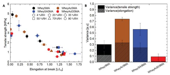
Fig. 6 (A) Elongation at break and ultimate tensile strength of copolymers equilibrated at relative humidity levels ranging from 4–90% RH. Copolymers are color coded based on the type of protein modification, and the equilibration conditions are noted with different marker shapes. Copolymers with small mechanical property variations with humidity are clustered closer together. (B) Data clustering from 20-90% RH determined as the variance.
