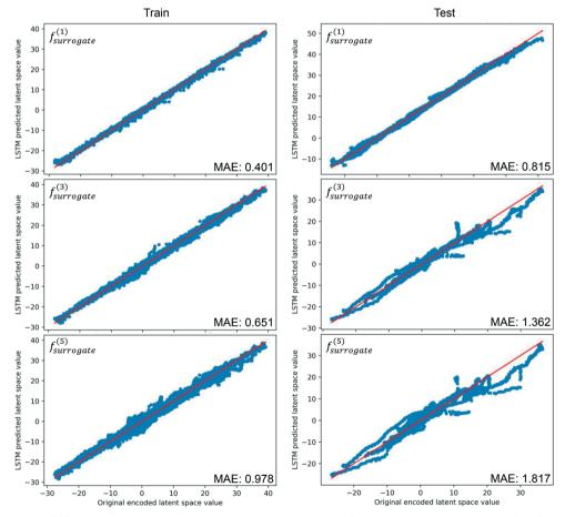
Fig. 6 Results of iterative S2S estimations on the widest span latent variable, MAE is computed by comparing the differences between the estimated and the true latent variables.
