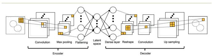
Fig. 2 Encoding-decoding layout of the constructed CAE
