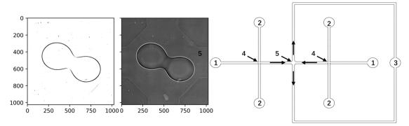
Fig. 1 Scheme of the microfluidics device (right): 1 - inlets for dispersed phase, 2 - inlets for continuous phase, 3 - outlet, 4 - X-junctions for drop formation, 5 - coalescence chamber; event of drop coalescence in the coalescence chamber: the processed image and the original image (left).
