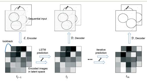
Fig. 3 Schematic of iterative LSTM estimation procedure.
