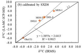
Fig. 8 Carbon isotopic fractionation of different carbonate minerals including calcite, dolomite, magnesite and siderite using fs-LA-MC-ICP-MS in two different analytical sessions (a and b).  $\delta^{13}$ C obtained by fs-laser ablation is a function of that obtained by IRMS, represented by the dashed line, applying SXD8 calcite as a calibration standard. The solid line is a 1:1 reference line.
