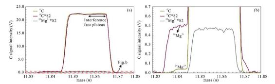
Fig. 4 Peak shapes for <sup>12</sup>C and <sup>13</sup>C obtained from MGS-1. Interference of doubly charged Mg ions superimposed on the low mass shoulder of <sup>12</sup>C and  $^{13}$ C, which leaves the high mass shoulder as the interference free plateau. Signal intensities of  $^{13}$ C and  $^{25}$ Mg<sup>2+</sup> were multiplied by 82 to match the signal intensity of <sup>12</sup>C.
