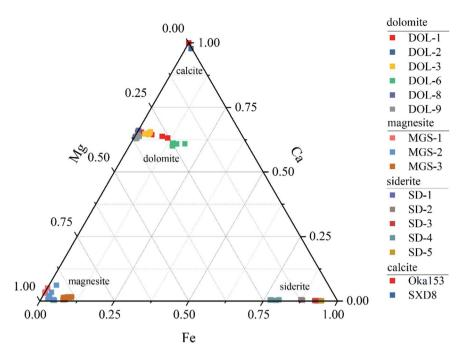
Fig. 1 Major-element variations of different carbonate matrices (dolomite, magnesite, siderite and calcite).
