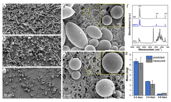
Fig. 4 SEM images of the NMP particles on the membrane, released during 0–2 (a and d), 2–4 (b), and 4–6 (c and e) days of ageing; (f) IR spectra of neat PE, NMPs formed during 0–2 days of ageing, and neat PCL and (g) predicted and measured mass of the NMPs formed during different ageing periods. The inset in d and e shows typical NPs released during ageing.
