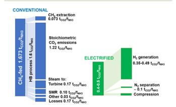
Fig. 7 Sankey diagram comparing CO<sub>2</sub> emissions breakdown for conventional HB process and the electrified version, where H2 is produced by electrolysis then used in the HB thermocatalytic process. Based on the data reported in ref. 168.
