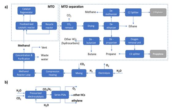
Fig. 1 Simplified block scheme of the process to synthesize olefins from  $CO_2$ : (a) route A *via* producing  $H_2$  by electrolysis followed by thermocatalytic synthesis of methanol then converted to olefins by MTO process; (b) route B of direct production of ethylene by electrocatalytic conversion of  $CO_2$  and  $H_2O$ .
