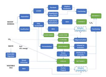
**Fig. 6** Overview of different possible routes to produce FFs-free aromatics as raw materials for the chemical industry. Surrounded by a broken line indicates technologies still to be developed. HDO indicates hydrodeoxygenation.
