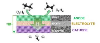
Fig. 5 Schematic illustration of the ethane to ethylene + H<sub>2</sub> coproduction on solid proton-conductive membranes in an electrochemical cell. Adapted ref. 65 with permission. PrBa<sub>0.5</sub>Sr<sub>0.5</sub>Co<sub>1.5</sub>Fe<sub>0.5</sub>O<sub>5+ $\delta$ </sub> (porous double perovskite, 30  $\mu$ m). BZVYYb =  $BaZr_{0.1}Ce_{0.7}Y_{0.1}Yb_{0.1}O_{3-\delta}$  (doped barium zirconate cerate, 10 µm). Ni-BZCYYb = NiO: BZCYYb 6:4 wt. Copyright © 2018, Royal Society of Chemistry.
