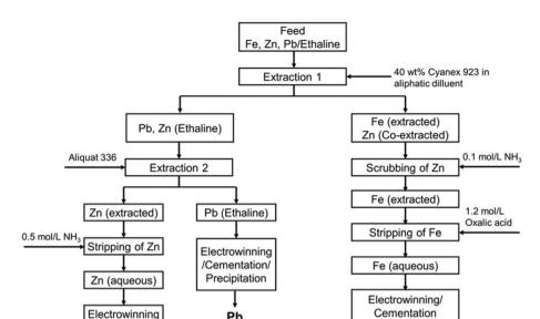
Fig. 16 Proposed flowsheet for the separation and recovery of Fe(III), Pb(II) and Zn(III) a mimicked jarosite waste stream. Reprint with permission from ref. 216, Copyright © 2020, Royal Society of Chemistry
