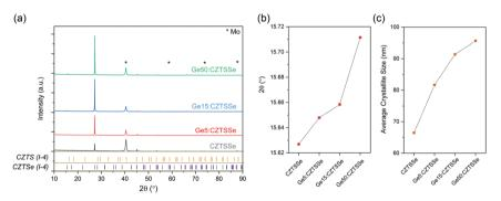
Fig. 2 (a) Structural analysis of CZTSSe films using XRD. XRD patterns of CZTSSe films with or without Ge along with the Bragg reflections of kesterite (I-4)  $Cu_2ZnSnS_4$  and  $Cu_2$ -ZnSnSe<sub>4</sub>. (b)  $2\theta$  shift of the (002) peak and (c) average crystallite sizes of (002) orientation CZTSSe films with respect to the Ge amount.
