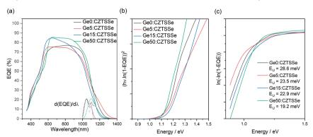
Fig. 7 (a) EQE for CZTSSe films with and without Ge. (b) Normalised first derivative of EQE with respect to wavelength at the CZTSSe absorption edge. (c) Urbach energy determination of CZTSSe from the sub-bandgap absorption region.
