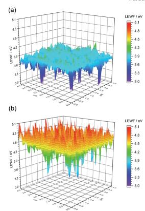
Fig. 9 LEWF maps showing the electronic terrain for the (a) CZTSSe and (b) Ge50:CZTSSe surfaces measured after heat treatment at 300 °C in UHV for 1 hour.
