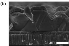
Fig. 3 Cross-sectional scanning electron micrograph of a complete solar cell device (SLG/Mo/(Ge)CZTSSe/CdS/i-ZnO/ITO) fabricating using (a) no Ge doping and (b) a 50 nm Ge underlayer.
