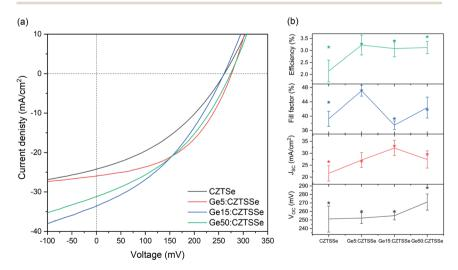
Fig. 6 CZTSSe device performance (a). J-V characteristics under a simulated AM1.5G spectrum and (b) statistical analysis of the performance parameters:  $V_{\rm OC}$ ,  $J_{\rm SC}$ , fill factor and conversion efficiency, showing the standard deviation.
