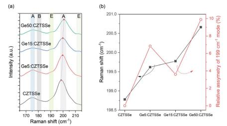
Fig. 4 (a). Raman spectra of CZTSSe films with or without Ge under 633 nm excitation. (b) Relative shift and asymmetry of the 199 cm<sup>-1</sup> peak measured for the CZTSSe films with and without Ge.
