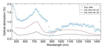
Fig. 1 The optical absorption of the NiO film with a thickness of 40 nm at wavelengths between 450 nm and 1450 nm. The circles represent the experimental data obtained from visible-infrared spectroscopy measurements. The sharp drop at 860 nm is due to the change of photodetector in the measurement. The dashed black and red lines denote the calculated optical absorption using the reported absorption coefficient in ref. 22 and 23, respectively.
