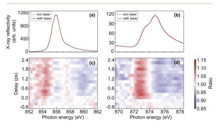
Fig. 3 (a and b) X-ray reflectivity spectra of NiO at the nickel  $L_{2,3}$ -edges. The dashed black and solid red lines represent the spectra acquired at time delays longer than 400 fs without and with laser excitation, respectively. (c and d) The ratio map as a function of delay and photon energy at the nickel  $L_{2,3}$ -edges.
