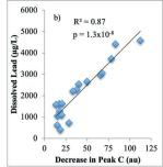
Fig. 5 Correlation between dissolved lead release and the decrease in humic-like a) peak A (Ex/Em = 250 nm/461 nm) and b) peak C (Ex/Em = 340 nm/457 nm) fluorescence intensities in arbitrary units (au) upon stagnation in the test pieces measured using FEEM. The data plotted is for TP2[pH+/DIC-/Hard-/NOM+], TP3[pH-/DIC+/Hard-/NOM+], TP5-[pH-/DIC-/Hard+/NOM+], TP8[pH+/DIC+/Hard+/NOM+], TP9[pH0/DIC0/Hard0/NOM0] and TP10[pH0/DIC0/Hard0/NOM0] in weeks 12, 16 and 20.
