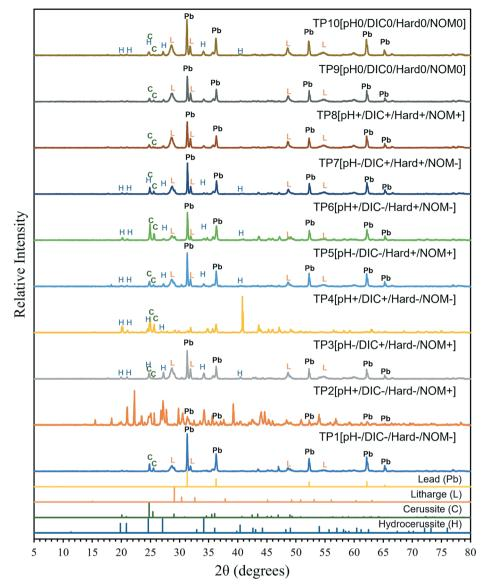
Fig. 6 XRD patterns obtained from the surface of the lead pipes for a range of  $5^{\circ}$  to  $80^{\circ}$   $2\theta$ . The patterns at the bottom are the reference patterns of the solids that had peaks identified in the samples.
