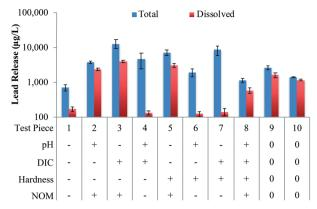
Fig. 2 Total and dissolved lead release from the test pieces. Total lead was measured from the weekly composite samples over the entire 20 week study. Dissolved lead was measured from the samples collected after the final 48 hour stagnation event in weeks 4, 8, 10, 12, 14, 16, 19 and 20. Bars represent average values and error bars represent the 90% confidence intervals.
