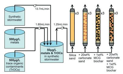
Fig. 1 Experimental setup of the column flow-through experiments with synthetic stormwater at pH 7.5 containing metals (Cd, Cu, Ni, Pb, Zn, each 50  $\mu$ g L<sup>-1</sup>) and TrOCs (1*H*-benzotriazole, atenolol, dicamba, diuron, fipronil, mecoprop, terbutryn, each 50  $\mu$ g L<sup>-1</sup>). The synthetic stormwater contained inorganic constituents and 5 mg C L<sup>-1</sup> DOC.
