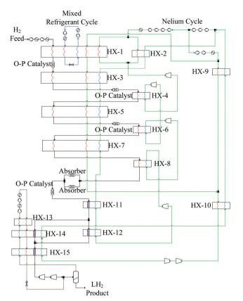
Fig. 8 Process block diagram for IDEALHY project.
