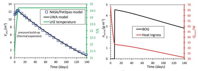
Fig. 16 Change of liquid hydrogen stored volume and boil-off gas rate over time in a 12.5 m<sup>3</sup> storage tank. Symbols correspond to the literature values while solid curves correspond to the value calculated using the model developed at the University of Western Australia (UWA).
