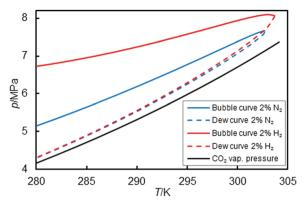
Fig. 11 Dew and bubble curves of impure  $CO_2$  in comparison with the vapour-pressure curve of pure  $CO_2$ . Equation-of-state model fitted to experimental data, adapted from ref. 206.
