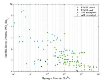
Fig. 5 The dependency of specific energy demand on the production rate today. Based on Smolinka. 150
