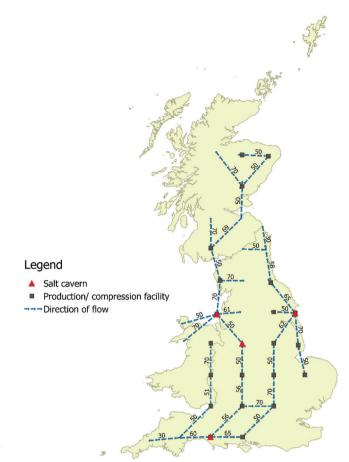
Fig. 12 Transmission of  $H_2$  to supply peak heat demands for Great Britain based on Sunny et al. <sup>125</sup> The direction of transmission is illustrated with the numeric labels representing the average operating pressure of the transmission line measured in bar. Salt caverns and production facilities dispense  $H_2$ , and booster compressors increase the transmission pressures to satisfy periods of high demand.
