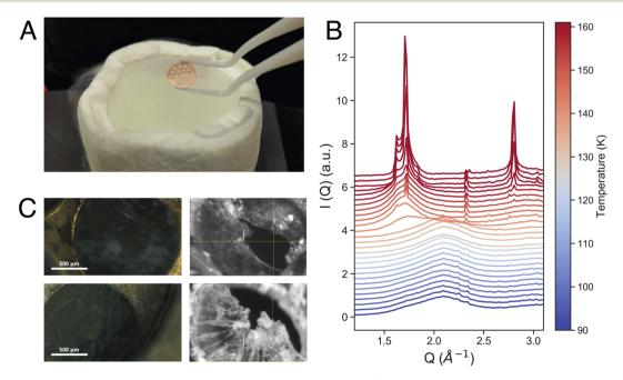
Fig. 1 A). Picture of the copper grid, inside of which the ice samples are formed. (B) Azimuthally integrated intensity in the WAXS range of an eHDA sample heated from 90 K to 160 K at 10 K min<sup>-1</sup>. (C) Four microscopy pictures of different amorphous ice samples.
