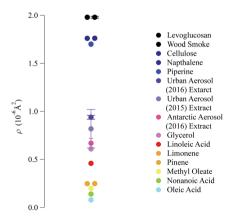
Fig. 2 Comparison of the neutron scattering length density for the films formed with material extracted from the aerosol filters and the scattering length density of some common pure compounds. The neutron scattering length density of pure compounds are calculated from tabulated scattering lengths94 and estimated mass densities.
