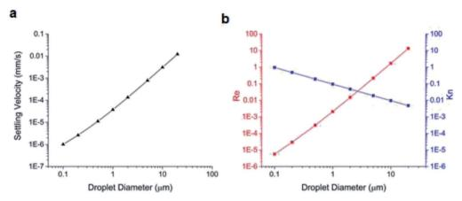
Fig. 2 (a) Calculated settling velocities of aerosols of varying sizes using Stokes—Cunningham law. (b) The Reynolds number (Re) and Knudsen number (Kn) of droplets of varying sizes. At Kn < 10, the Stokes—Cunningham law is the most applicable first-principle relationship to calculate settling velocity.
