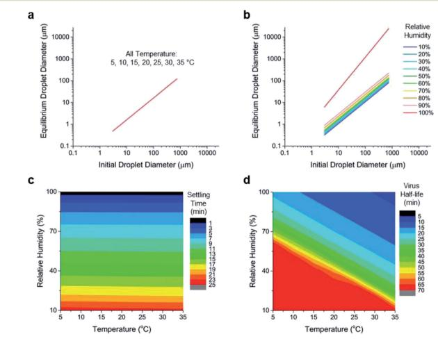
Fig. 3 Evaporated aerosol sizes derived from the Köhler equation based on an initial size at different ambient (a) temperatures at 50% relative humidity and (b) relative humidity at 25  $^{\circ}$ C. (c) Calculated settling times obtained from the empirical model using 6  $\mu$ m as the initial droplet size and (d) viral viability at different ambient temperatures and relative humidity.
