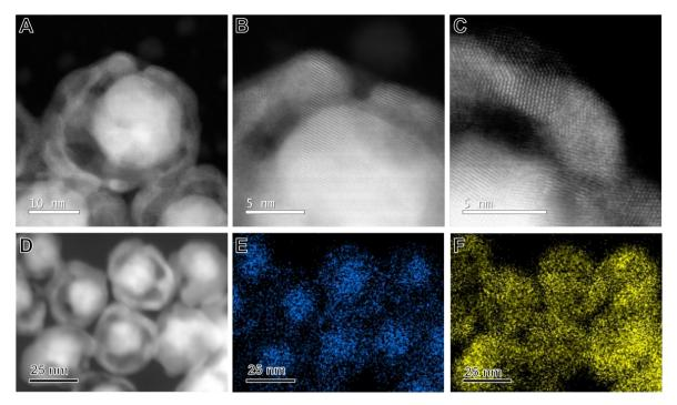
Fig. 2 (A–D) STEM-HAADF images of the Au@AgAu NRs, in which the brightest contrast from the Au core results from its higher Z (atomic number) as  $Z_{Au} > Z_{Ag}$ . (E and F) Corresponding EDS elemental maps of (E) Au (blue) and (F) Ag (yellow) of the region shown in (D).
