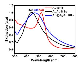
Fig. 3 Normalized UV/Vis extinction spectra were recorded from aqueous suspensions containing Au NPs (red trace), AgAu NSs (black trace), and Au@AgAu NRs (blue trace).
