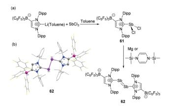
Fig. 20 (a) Synthesis of diantimony compound 62 from NHC-stabilized dichlorostibane, 61; (b) solid-state structure of 62.
