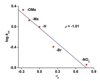
**Fig. 8** Hammett plot of  $\log k_{\rm rel}$  vs.  $\sigma_{\rm p}$  for the reaction of **8** with *p*-substituted thioanisoles.
