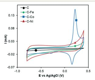
Fig. 6 Cyclic voltammograms in  $N_2$ -saturated KOH solution at 1000 rpm and 50 mV s<sup>-1</sup> of C, C–Fe, C–Co and C–Ni.
