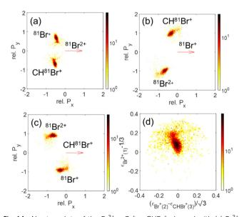
Fig. 14 Newton plots of the  $Br^{2+} + Br^{+} + CHBr^{+}$  channel with (a)  $Br^{2+}$ , (b)  $Br^{+}$ , or (c)  $CHBr^{+}$  as the reference fragment. (d) Dalitz plot for the same fragmentation channel.
