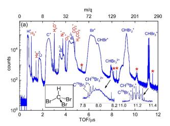
Fig. 2 Ion time-of-flight (TOF) spectrum of CHBr<sub>3</sub> exposed to intense NIR laser pulses (the mass to charge ratio, m/q, is shown on the top axis) along with a cartoon geometry of CHBr3 shown in the inset. Residual gas peaks are labeled in red. The '\*' labeled peaks are unidentified
