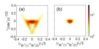
Fig. 11 Dalitz plots for the  $Br^+ + Br^+ + CHBr^+$  channel: (a) all  $Br^+ + Br^+ +$ CHBr<sup>+</sup> events, (b) similar to panel (a) but with KE of each Br<sup>+</sup> fragment being smaller than 5.1 eV in order to select the contribution from concerted breakup (see text). The result of the CES for concerted breakup is shown as a green cross "x" symbol.
