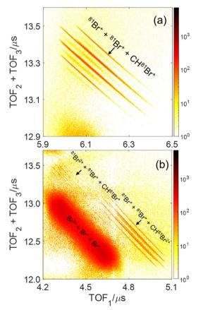
Fig. 5 Triple photoion coincidence (TRIPICO) plot of  $CHBr_3$  for the same laser conditions as the previous plots. The three-body breakup into (a)  $Br^+ + Br^+ + CHBr^+$ , and (b)  $Br^{2+} + Br^+ + CHBr^+$  and  $Br^+ + Br^+ + CHBr^{2+}$ , after subtraction of random coincidences.
